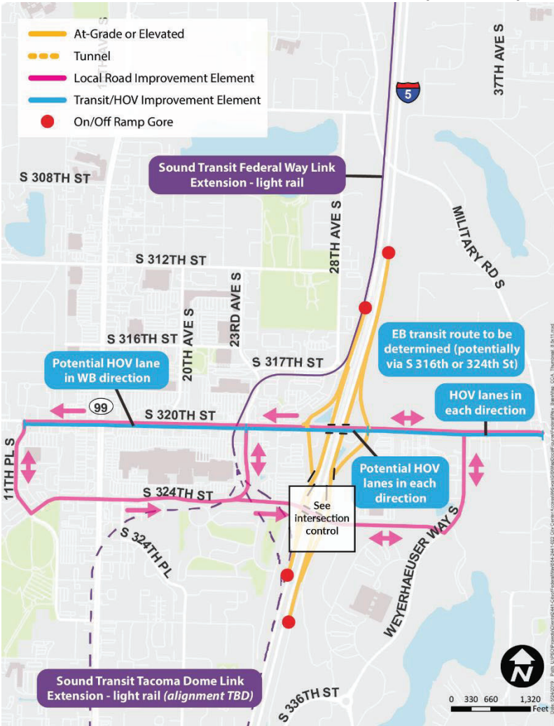
Exhibit 15. Arterial Couplet (2C) (Shown with the Grade Separated Interchange Alternative) – Level 2 Screening
